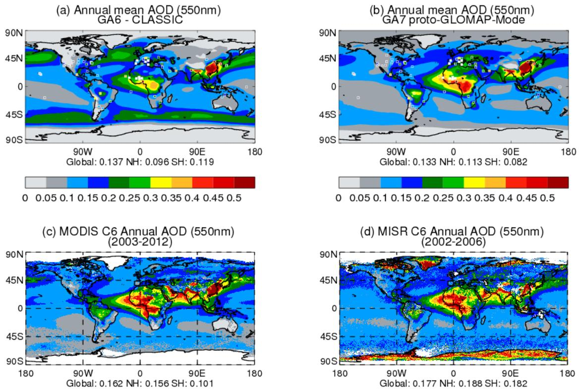
Figure 2: Annual mean AOD at 550nm in (a) GA6 CLASSIC simulation, (b) GA7 prototype simulation with GLOMAP-Mode, (c) MODIS and (d) MISR observations. Model simulations are taken from years 2002-2008 of a 20 year free-running AMIP simulation. Observations cover the period 2003-2012 for MODIS and 2002-2006 for MISR.
