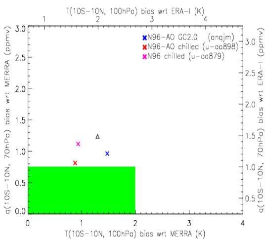
Figure 1: Error in tropical specific humidity at 70hPa (y-axis) against error in temperature at 100hPa (x-axis). GA6 and GA7 are the black triangle and pink cross respectively. GC2 and GC3 are the blue cross and orange cross respectively. The green box marks the desired error range for use of the model with interactive chemistry.
